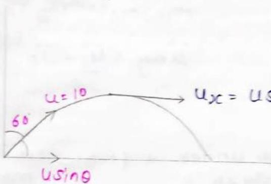
$$\begin{aligned} u_x &= u \sin \theta = 10 \times \sin 60^\circ \\ &= 10 \times \frac{\sqrt{3}}{2} \\ &= 5\sqrt{3} \text{ ms}^{-1} \end{aligned}$$
