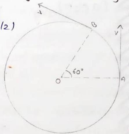
Que - A body moving in a uniform circular motion with speed  $v$ , the magnitude of change in its velocity after it rotates by an angle  $120^\circ$  is
