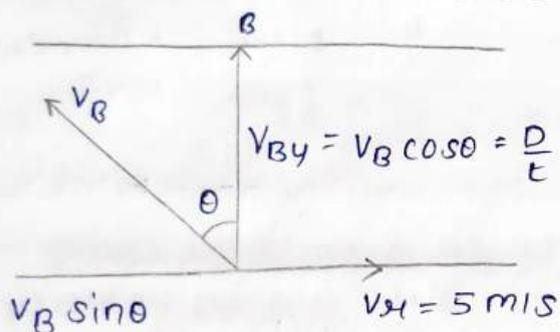
$$v_{By} = v_B \cos \theta = \frac{D}{t} = \frac{60}{5} = 12 \text{ m/s} \quad \text{--- (i)}$$
